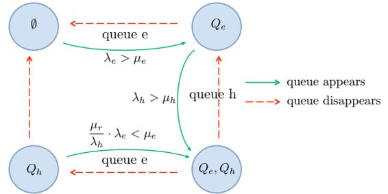
Fig. 3: State transitions in the off-ramp model. The four states  $\emptyset$ ,  $Q_e$ ,  $(Q_e, Q_h)$  and  $Q_e, Q_h$  correspond respectively to the cases (a), (b), (c) and (d) from figure 2.
