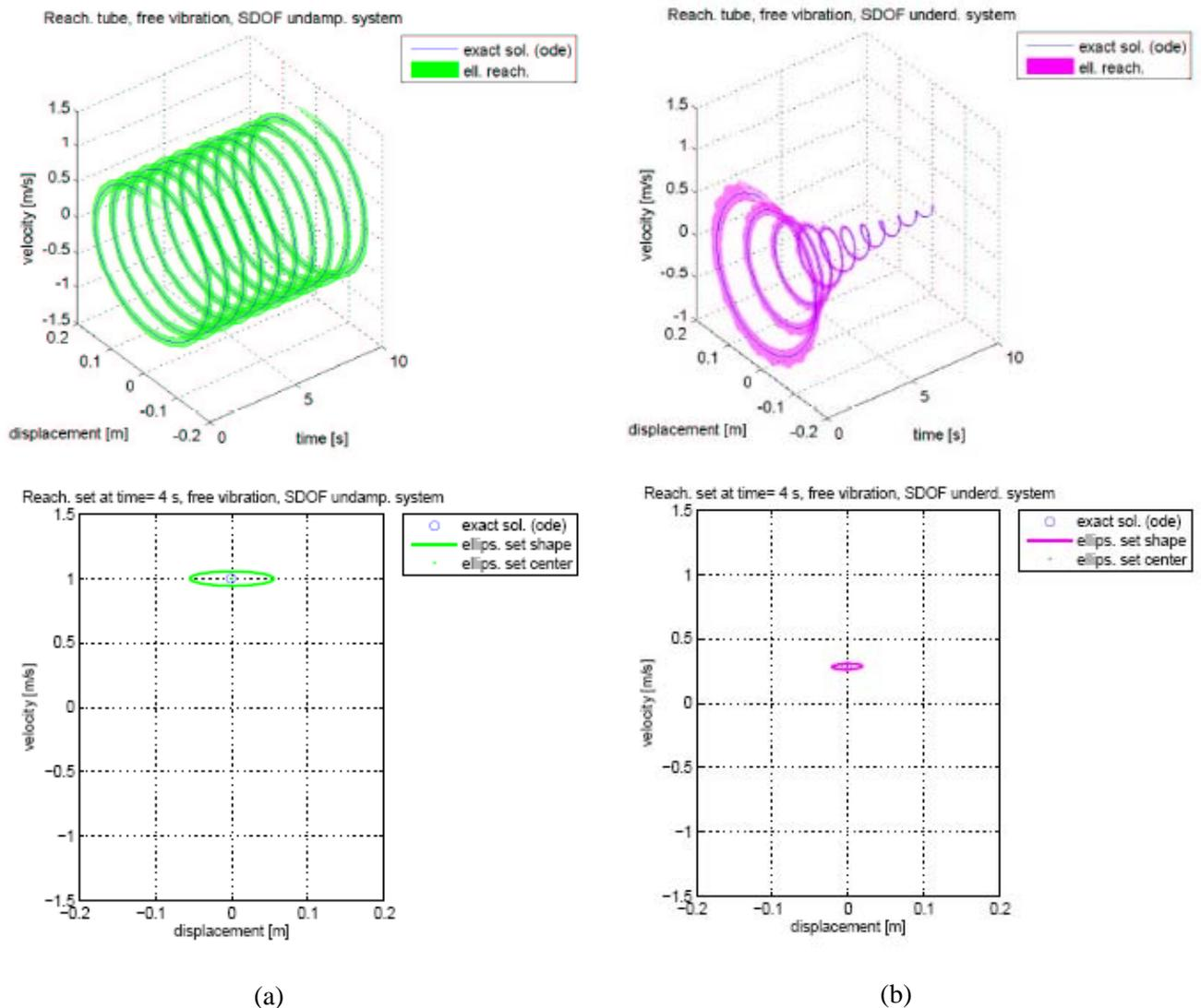
Figure 2. Free vibration response and the ellipsoidal reachable tube for an undamped (a) and 2%-damped (b) SDOF system.
