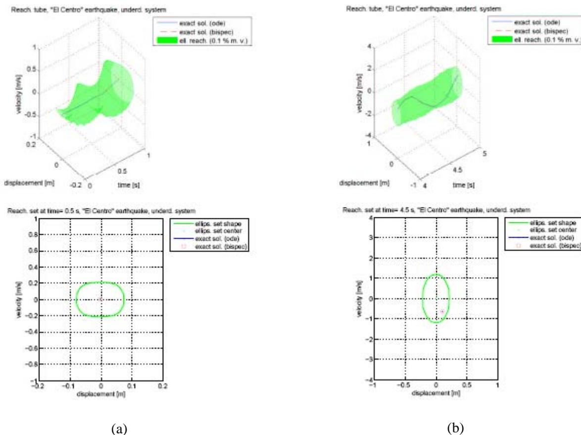
Figure 4. Reachable tube of the response of the 2%-damped linear elastic SDOF system to 1940 NS El Centro ground motion for the  $[0,1]$ sec (a) and  $[4,5]$ sec (b) time interval and reachable sets at  $t = 0.5$ sec and  $t = 4.5$ sec instances of the response.
