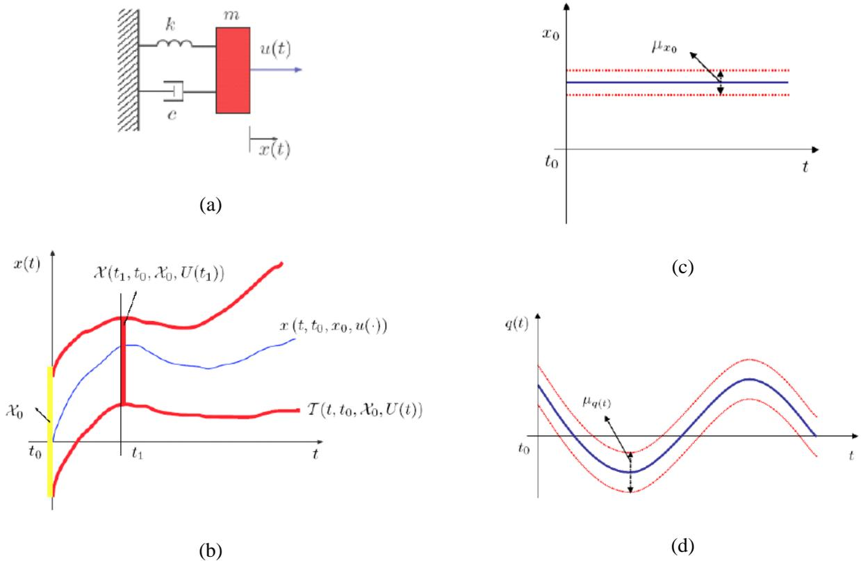
Figure 1. (a) SDOF system; (b) Definition of reachable set and tube; (c) Disturbance in the initial state of the SDOF system; and (d) Disturbance in the SDOF system excitation.
