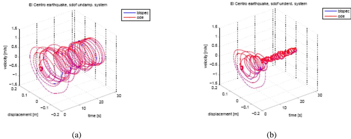
Figure 3. SDOF system response to the 1940 NS El Centro earthquake record: (a) undamped; (b) 2% damped.
