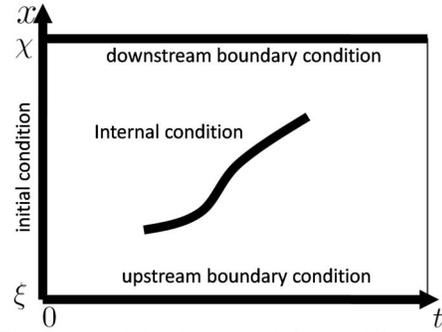
Fig. 1. Illustration of the domains of the possible value conditions used to construct the solution of the Moskowitz HJ PDE.
