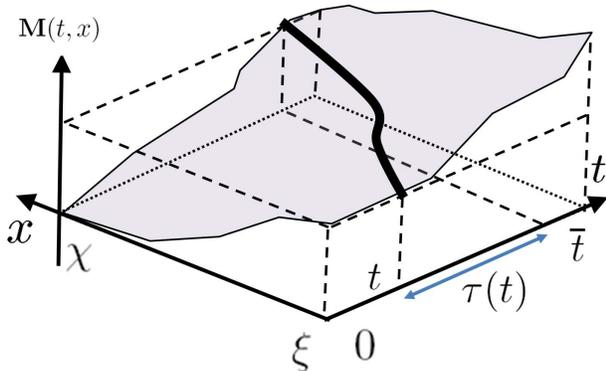
Fig. 2. **Isopleth of the Moskowitz function.** The projection of this level set in the  $(t, x)$  plane is the trajectory of vehicle  $\bar{\mathbf{M}}$ .
