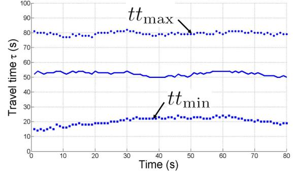
Fig. 5. Estimation of the travel time function using boundary conditions functions only. The horizontal axis represents the time  $t$ . The exact value of the travel time function  $\tau(\cdot)$  is represented using a solid line. The upper and lower bounds on  $\tau(t)$  obtained by solving problem (38) and using definition 4.1 are represented by circles and squares respectively.
