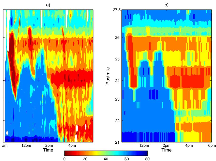
FIGURE 5. Velocity contour map (in mph) using a) vehicle trajectories and Edie's speed definition, b) 17 loop detector stations.
