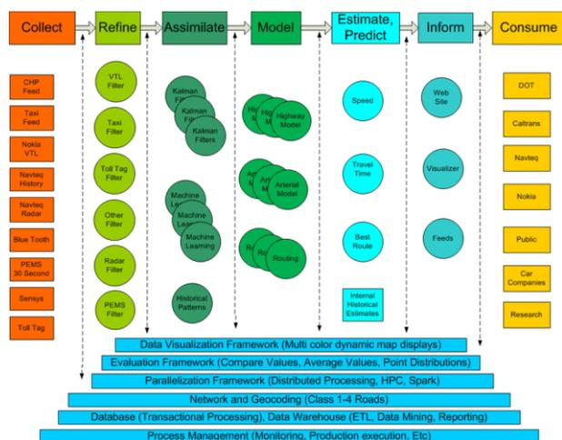
**Figure 1 *Mobile Millennium*:** A variety of data feeds from different data sources is processed and fed in real-time to statistical and model-based estimation algorithms. The real-time output of these algorithms is then broadcast to different classes of clients under the form of link travel-time distributions, velocity maps, and optimal routing policies.
