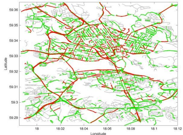
**Figure 2** Network links color-coded according to the number of taxi probes per link for the time period 8:00 to 8:15 AM during five weekdays from March 1 to March 5 2010. Green and red colors denote links with lower (<10) and higher (>=10) number of probes respectively. Gray lines are network links with zero number of probes.
