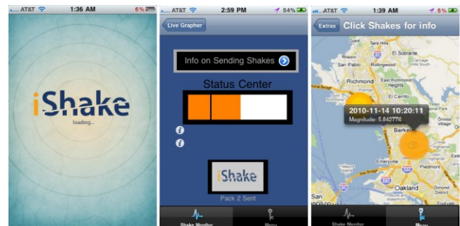
Figure 5. “Shake Monitor” interface and “iShake Map” generated on client application.
