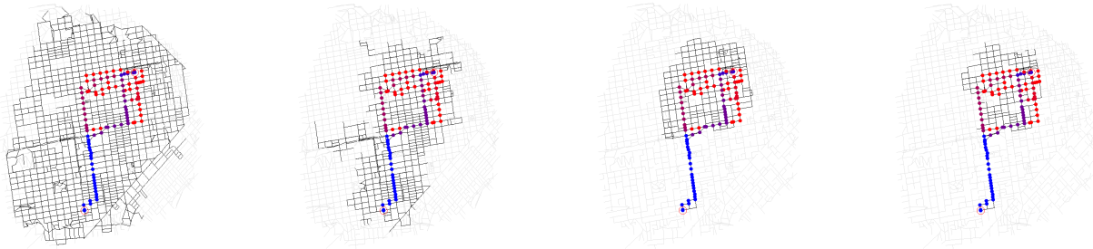
Figure 4: pruning of the San Francisco network for some source-destination pair. From left to right the pruning achieved using reach, directed-reach, arc-flags and the combination of reach with arc-flags. The colored nodes are the nodes that belong in the optimal policy and the color denotes the probability of the node being used, where blue indicates a high probability and red indicates a low probability. The source is in the bottom of the graph.
