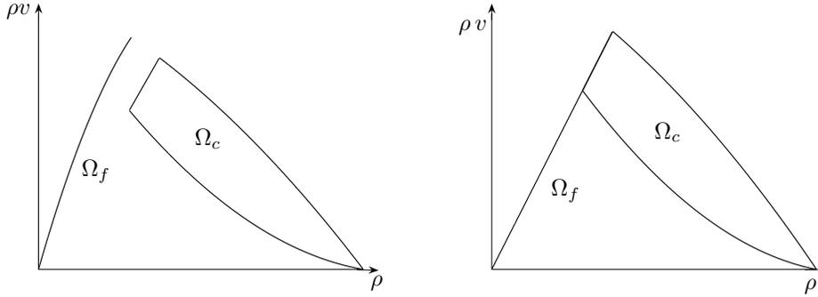
FIG. 3.2. *Different free-flow phases. Left: Fundamental diagram from the original Colombo phase transition model. Right: Fundamental diagram of the model derived in the present article in the particular case of a Newell-Daganzo flux-density relation for congestion at equilibrium.*
