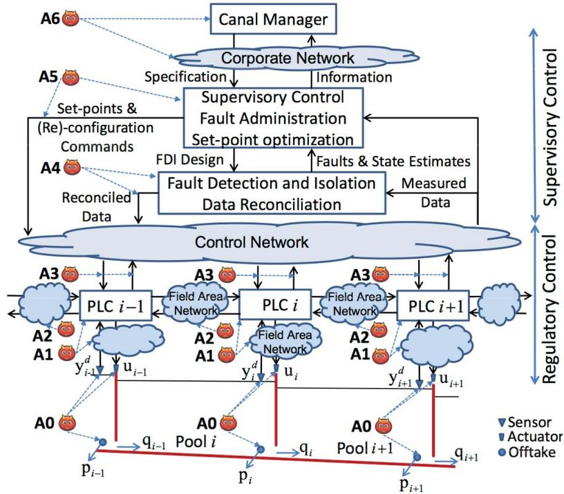
Fig. 1. Cyber attacks to hierarchical water SCADA systems.
